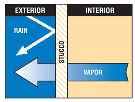
The Loxon system allows the coating to resist wind driven rain. It also allows the masonry structure to release moisture vapors without interfering with the adhesion and the performance of the coating.
